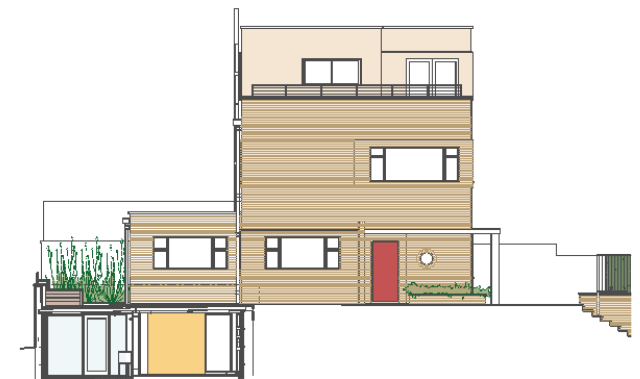
Proposed north-east elevation and part section
